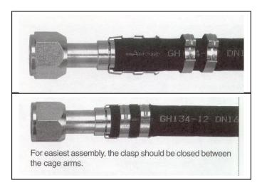
Step 7. Use the pliers to close the clips. The pliers should be positioned squarely on the clip connection points and should remain square during the closing of the clip.
